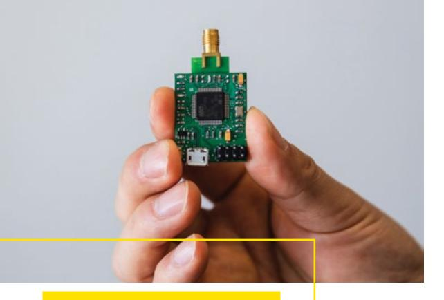
A wide area geospatial positioning system for underground environments that features high accuracy, robust design, inertial measurement, geomagnetic sensing and low energy Bluetooth communications. Applicable in environments where GPS is unavailable.
