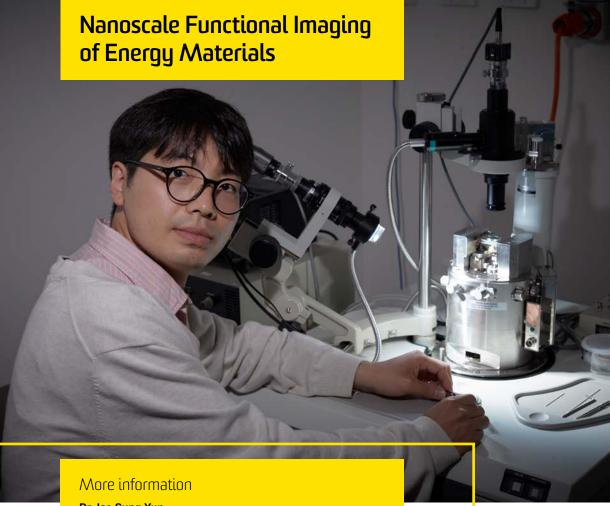
Understanding the nanoscale properties of energy materials is critical in optimising their performance. Nanoscale functional imaging, using the atomic force microscope to measure local electrical and structural behaviour to gain deeper insight, is superbly suited for this purpose.
