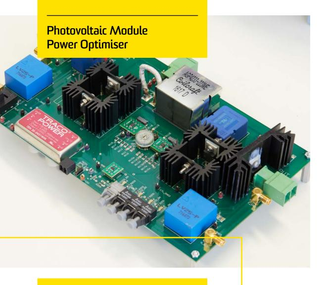
A low-cost universal converter that can act as either a power optimiser or a micro-inverter for photovoltaic (PV) modules would maximise the energy output of photovoltaic systems by constantly extracting the maximum power from each photovoltaic panel separately.
