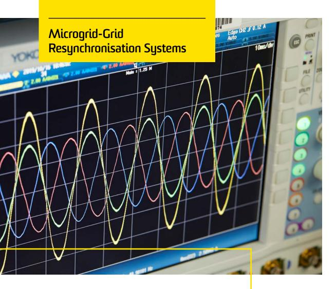
A resynchronisation system has been developed to bring the voltage, phase and frequency of a microgrid back into alignment with the main grid in the event of a fault on the distribution line.
