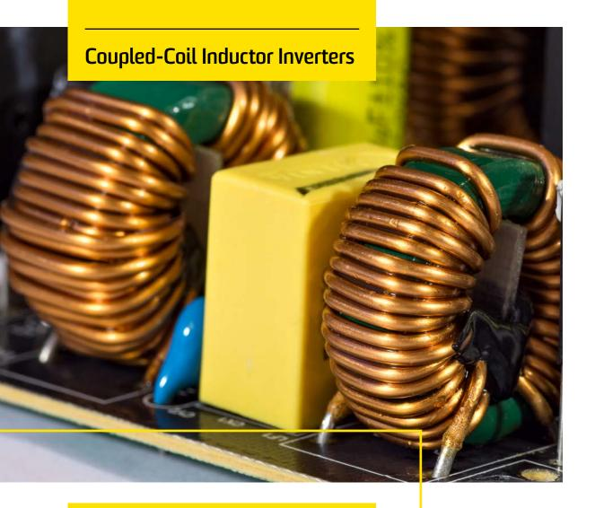
Producing multi-level output voltage from just two fast-switching semiconductors by using a coupled inductor. This frees the inverter from dead-time and greatly reduces low-order harmonics.
