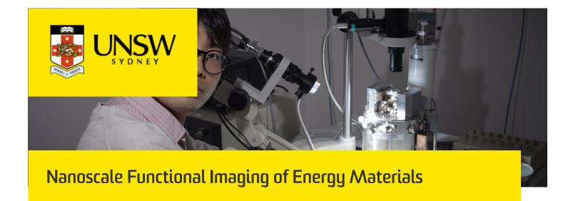
Understanding the nanoscale properties of energy materials is critical in optimising their performance. Nanoscale functional imaging, using the atomic force microscope to measure local electrical and structural behaviour to gain deeper insight, is superbly suited for this purpose.
