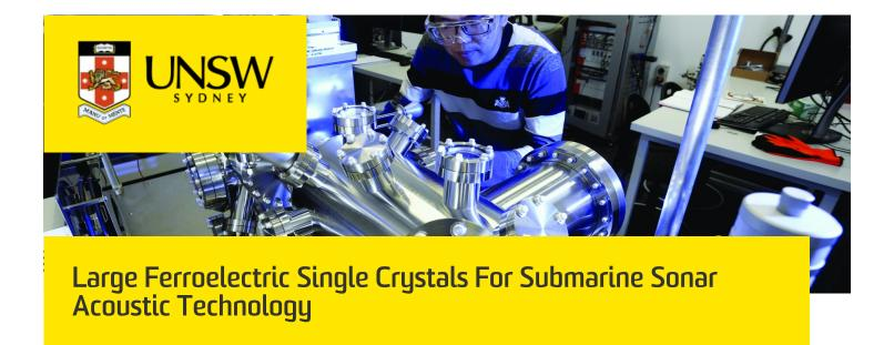
Mirror furnace systems are used to produce very uniform high-quality single crystals of ferroelectric materials for use in sensors including those used in submarine sonar systems.
