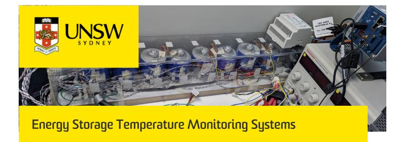
In an energy storage string or module consisting of a number of cells, a significant variation in temperature distribution can exist. However, monitoring the whole module temperature is often hindered by hardware and cost limitations and, typically, only a limited number of temperature sensors are employed.
