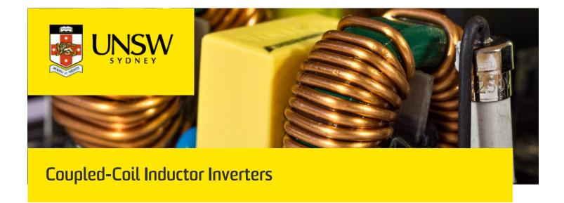
Producing multi-level output voltage from just two fast-switching semiconductors by using a coupled inductor. This frees the inverter from dead-time and greatly reduces low-order harmonics.
